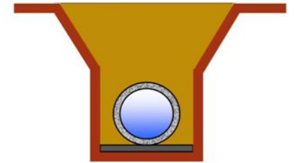
RCP TYPE 4 INSTALLATION
